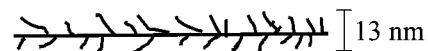
Fig. 7. Schematic drawing showing a branched pore. The diameter of the pores measured using TEM may be the space taken up by a pore and its branches.
