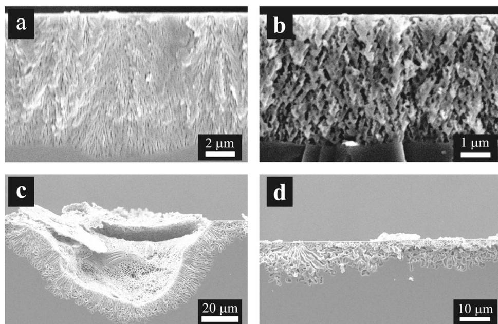
**Figure 3.** Side views of GaP samples etched in 1 M HNO<sub>3</sub> at potentials of 13 V (a), 15 V (b), and 17.6 V (c, d). Because at 17.6 V the morphology depended strongly on the location on the sample, two pictures from different locations on the same sample are shown. Samples were etched until a charge density of 10 (a,b) or 5 (c,d) C/cm<sup>2</sup> was reached.
