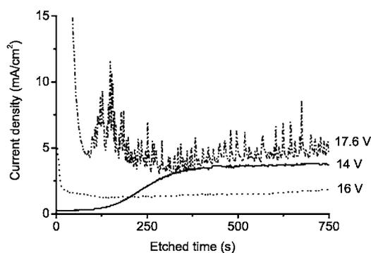
**Figure 2.** Current-time curves of n-type GaP etched at different potentials in 1 M HNO<sub>3</sub>.
